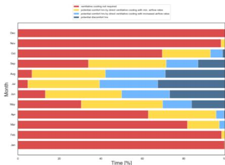
Light blue bars represent the percentage of time when ventilative cooling can potentially provide comfort.
