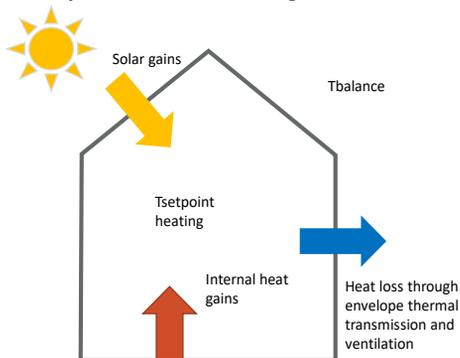
The **heating balance point temperature** is the outdoor temperature at which heat gains are equal to heat losses.
