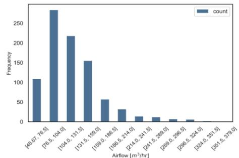
Frequency of the required airflow rates to keep building temperature within the comfort range.
