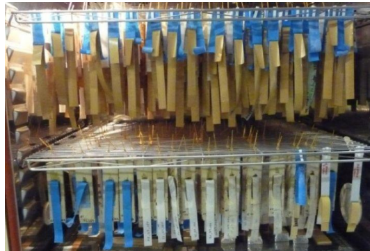
Accelerated ageing of bonding samples: Exposition to climate 65°C/80% relative humidity for 60 weeks in climate chamber at Fraunhofer IBP/University of Kassel, Germany
