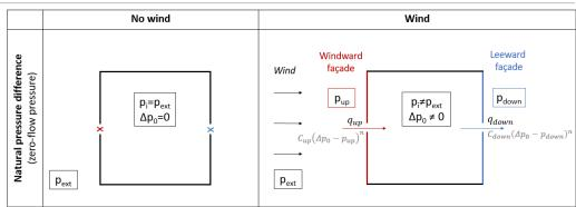
Equilibrium pressure:  $\Delta p_0 = p_i - p_{ext} = \frac{C_{up}^{\frac{1}{n}} p_{up} + C_{down}^{\frac{1}{n}} p_{down}}{C_{up}^{\frac{1}{n}} + C_{down}^{\frac{1}{n}}}$
