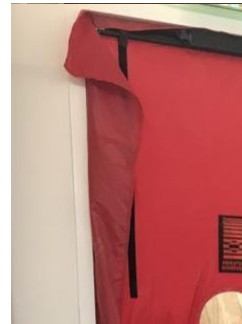
Fig. 3 DG1000 blast door air tightness test system
