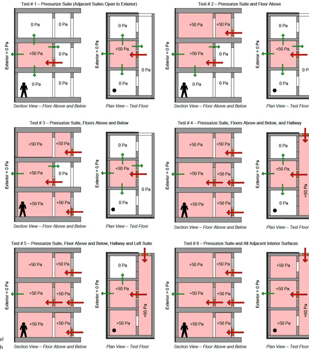
Figure 6.5: Balanced Fan Pressurization/Depressurization Method Schematic (Finch, 2007)
