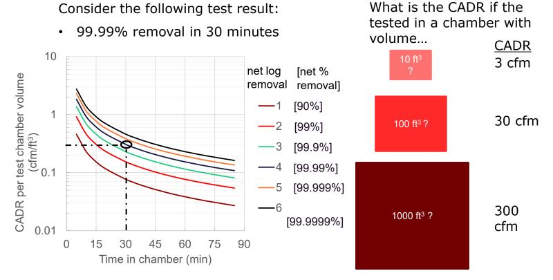
A wide range of CADRs can all claim 99.99% removal in 30 minutes, depending on test chamber volume
