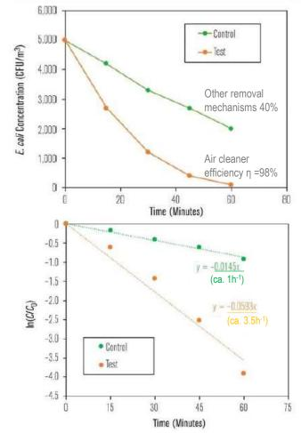
Removal rate difference in a 14.2 m<sup>3</sup> chamber: CADR=50-13=37 m<sup>3</sup>/h (2.5 h<sup>-1</sup>)
