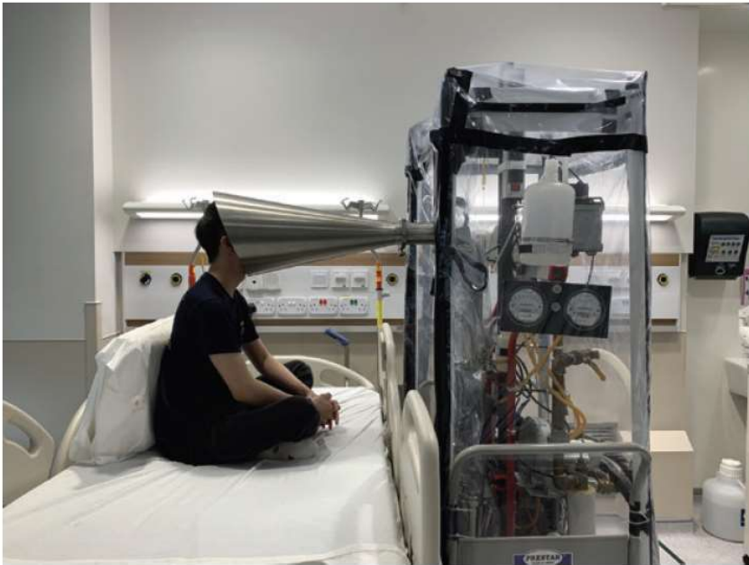
Figure 1. Schematic representation of expiratory sample collection using the G-II exhaled breath collector inside the COVID-19 patient room. Abbreviation: COVID-19, coronavirus disease 2019.
