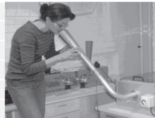
A test room for a in-duct air cleaner ( single-pass condition)
