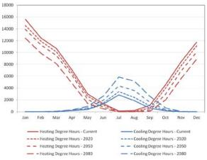
Figure 1 - Change in annual heating and cooling degree hours over time, Boston, MA
