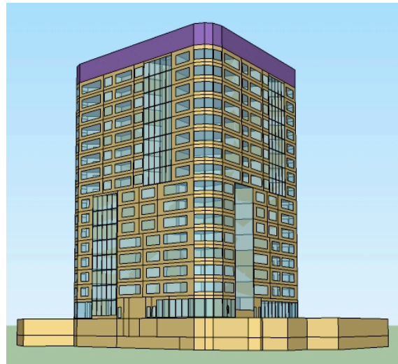
Figure 1: Geometry of the Energy Model in the OpenStudio Plugin for SketchUp
