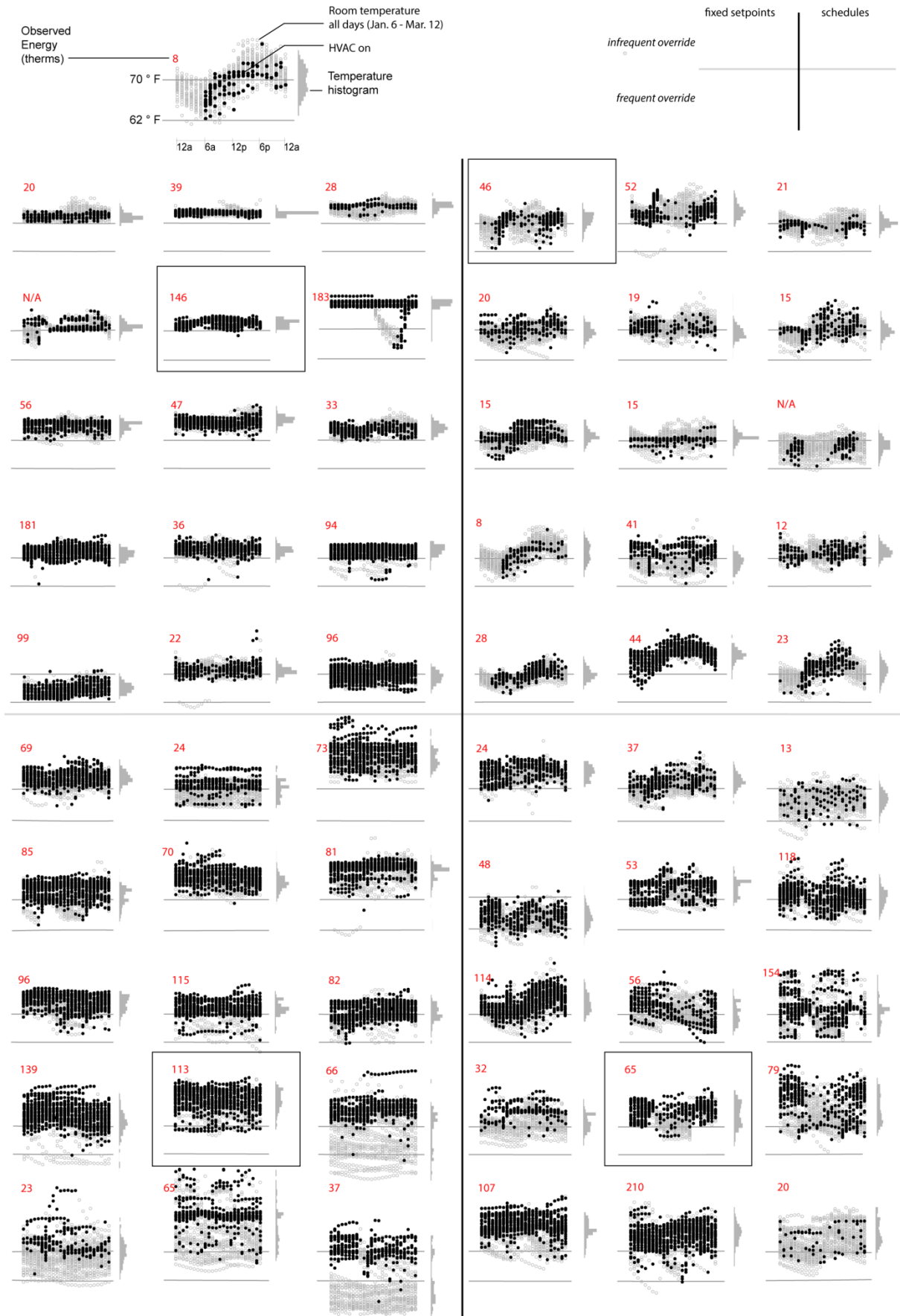
Figure 4 Temperature histories for all apartments. Black dots indicate the times that the heating system was on.
