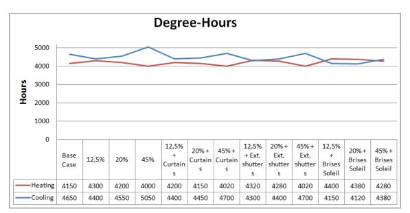
Chart 3 - Degree-hours of heating and cooling
