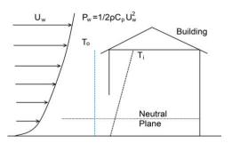
Figure 1 Pressure difference at the opening
