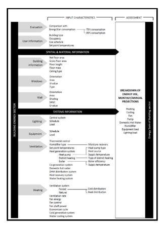
Figure 1: Description of BPAT+ Inputs and Outputs
