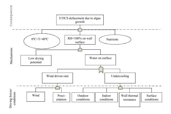
Figure 2 Fault Tree Analysis (FTA) for ETICS defacement (inspired in Pallin 2012).
