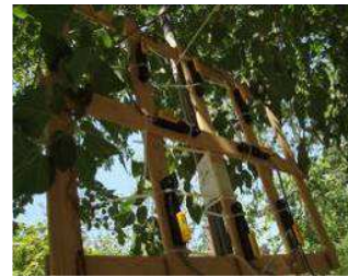
Figure 13: illuminance sensors located on the measurement grid.
