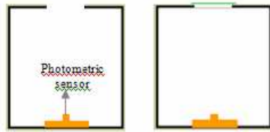
Figure 12: measurement diagram of transmittance without leaf (a) and with leaf (b).
