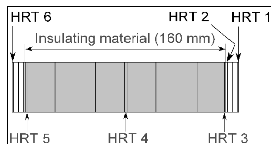
Fig. 9: Mesh applied to the insulated part of the vertical wall for the one-dimensional simulations and sensors location
