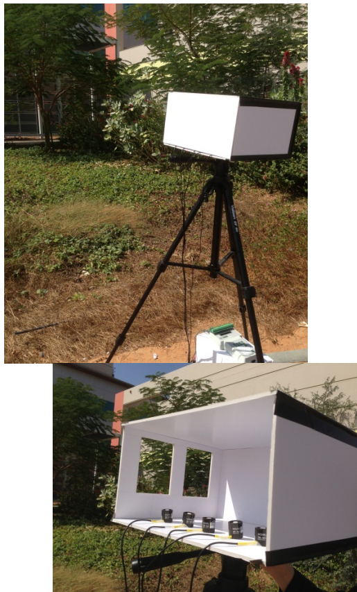
Figure 2 The experimental set up for measuring lux levels inside a real model in front of a tree.
