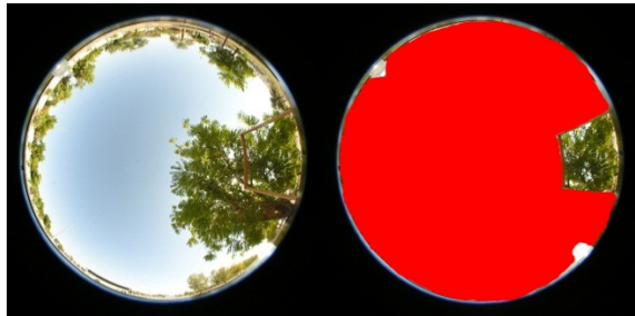
Figure 1 Hemispherical photograph of the real tree with the frame used to represent the window before and after image masking.
