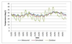
Figure 7 Measured and simulated bedroom temperatures of Unit 2
