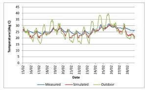
Figure 8 Measured and simulated bedroom temperatures of Unit 3
