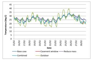
Figure 9 Changes in bedroom temperatures of Unit 1 due to design alterations
