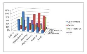
Figure 5 Occupant thermal sensations and ventilation/cooling strategies
