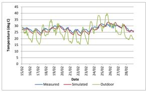
Figure 6 Measured and simulated bedroom temperatures of Unit 1
