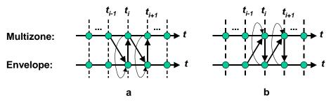
Fig. 3 Coupling schemes in time integration ( $t_i$  = current integration time point)
