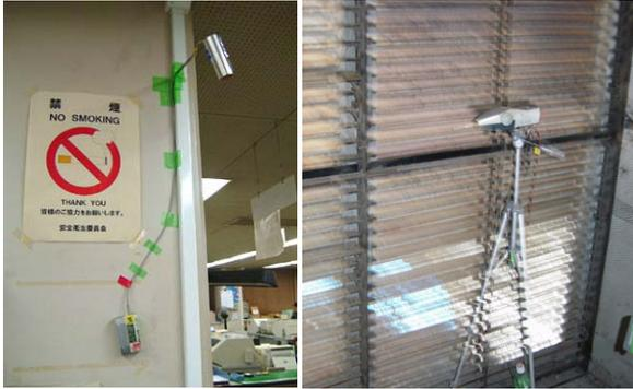
Figure 4 Photograph of measurement instruments (Left: Room air temperature and humidity, Right: Fresh air intake volume)
