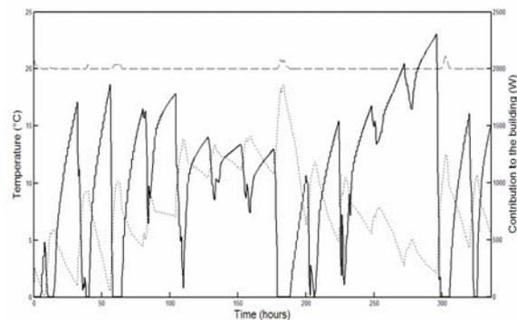
Figure 7: Evolution of the minimal heating need (Internal temperature, dashed line; External temperature, dotted line, heating power, solid line)
