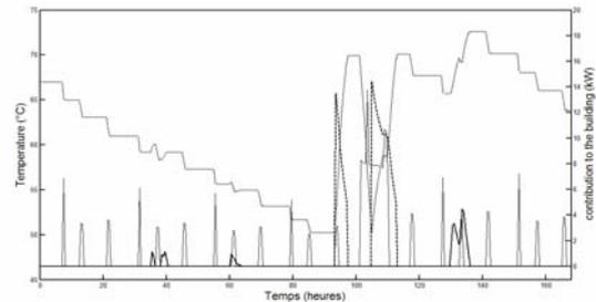
*Figure 8: Thermal state of the storage tank during a week of September (Average tank temperature, dotted line; Collector contribution, bolded solid line; Boiler contribution, dashed line; Thermal load, thin solid line)*
