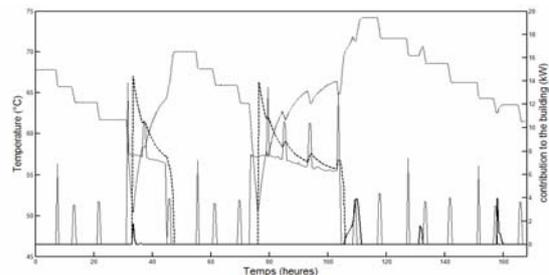
*Figure 9: Energetic state of the storage tank during a week of October (Average tank temperature, dotted line; Collector contribution, bolded solid line; Boiler contribution, dashed line; Thermal load, thin solid line)*
