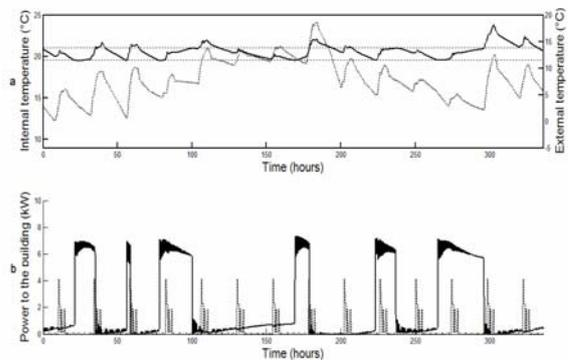
Figure 6 a: Evolution of the temperature in the building (Internal temperature, solid line; External temperature, dotted line)
