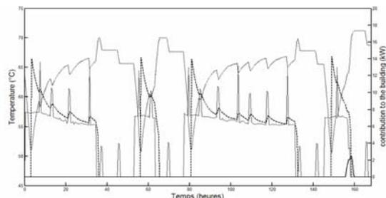
*Figure 10: Energetic state of the storage tank during a week of January (Average tank temperature, dotted line; Collector contribution, bolded solid line; Boiler contribution, dashed line; Thermal load, thin solid line)*
