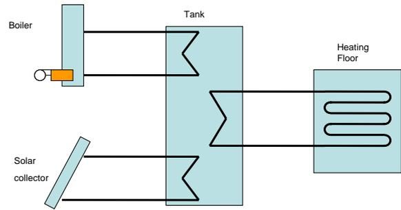
Figure 2: overview of the hydraulic net
