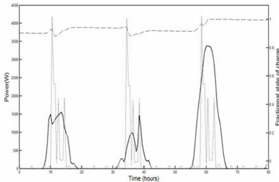
Figure 4: Electrical consumption and production with favourable weather conditions (Electrical consumption, dotted line; Photovoltaic production, solid line; Battery state of charge, Dash-dot line)
