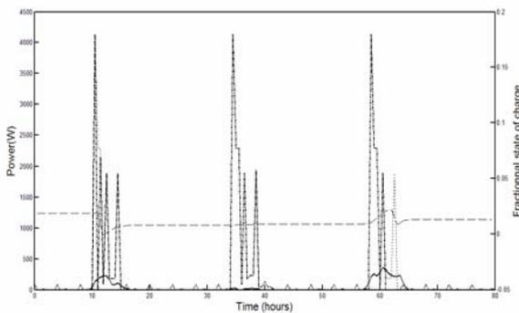
Figure 5: Electrical consumption and production with unfavourable weather conditions (Electrical consumption, dotted line; Photovoltaic production, solid line; Grid contribution, dashed line; Battery state of charge, Dash-dot line)
