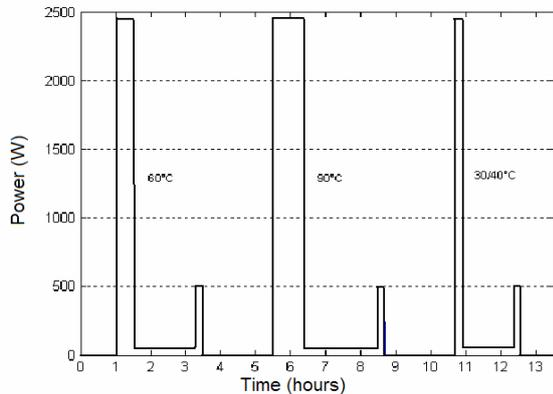
Figure 3: consumption profiles for a washing machine
