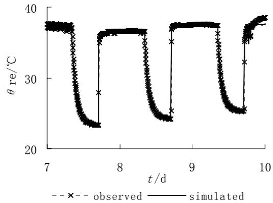
Fig.3 measured and calculated return water temperature
