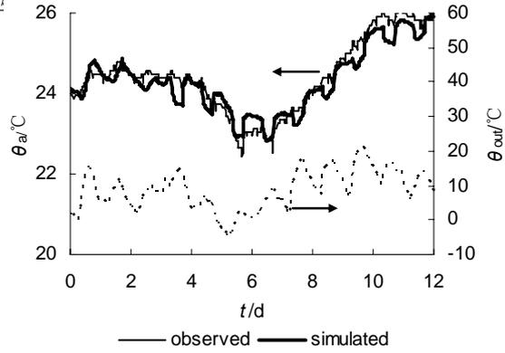
Fig.2 measured and calculated room temperature
