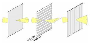
Fig. 5 - isotropic, horizontal and vertical geometry
