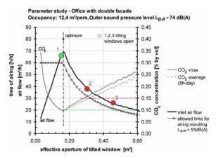
Fig. 8 – indoor air quality versus effective aperture in case of limited indoor sound pressure level
