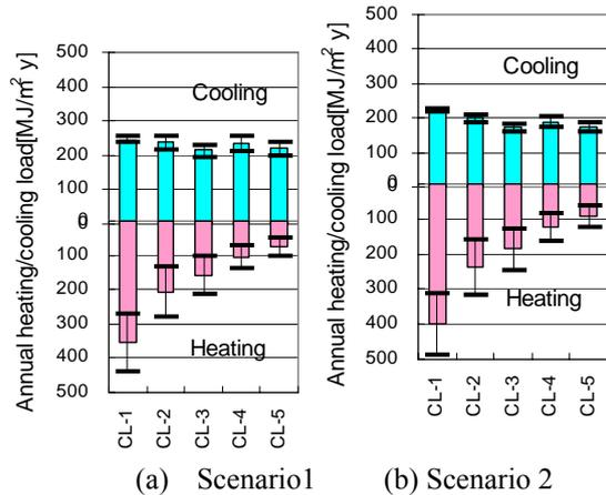
Figure 10. Simulated annual cooling and heating loads per unit floor area (CL-1~5 indicates office class 1~5 shown in Table 2)
