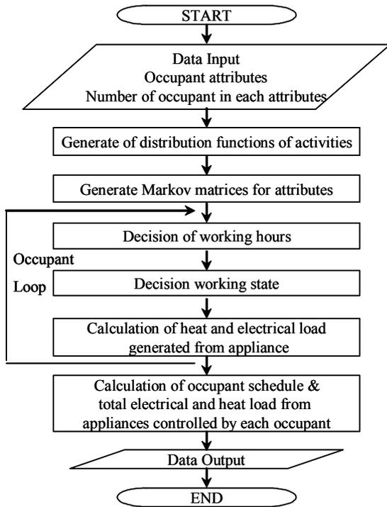
Figure 5 Flowchart of occupant behavior model in an office.
