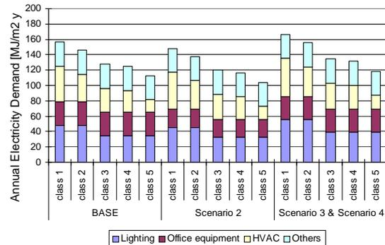
Figure 11. Simulated annual electricity demand per unit floor area of an office building ('class' indicates office class 1~5 shown in Table 2)
