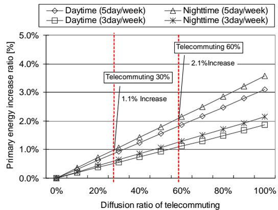
Figure 9. Relationships between diffusion ratio and primary energy consumption in a residential sector of Osaka City
