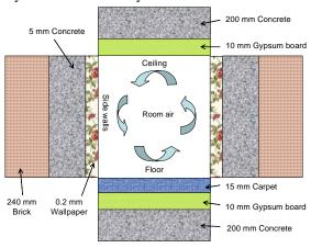
Figure 1 Structures of sidewalls, ceiling and floor
