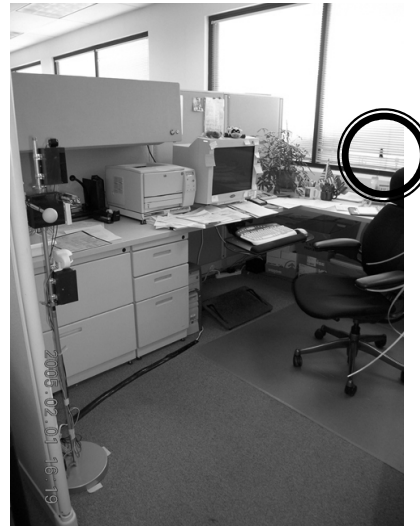
Figure 1 Location of the pyranometer that was mounted to the interior face of the window glass at approximately 1.22 m (4 ft) from the floor.
