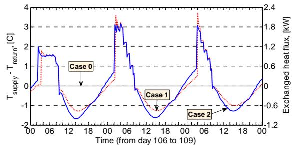
Figure 12 Total fluid temperature decline along the pipe loop within Zone A.
