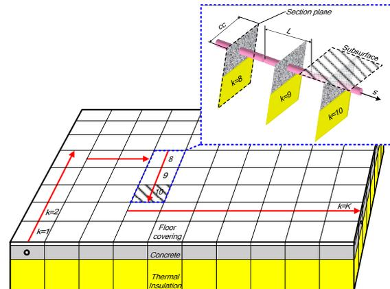
Figure 1 Illustration of space discretisation of a floor heating element with subsurfaces, section planes and pipe segments. The arrows indicate a conceivable pipe loop pattern. (Karlsson, 2006)
