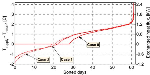
Figure 10 Total fluid temperature decline along the pipe loop within Zone A, illustrated as a duration diagram. The right hand axis represents the corresponding heat flux (fluid to concrete).
