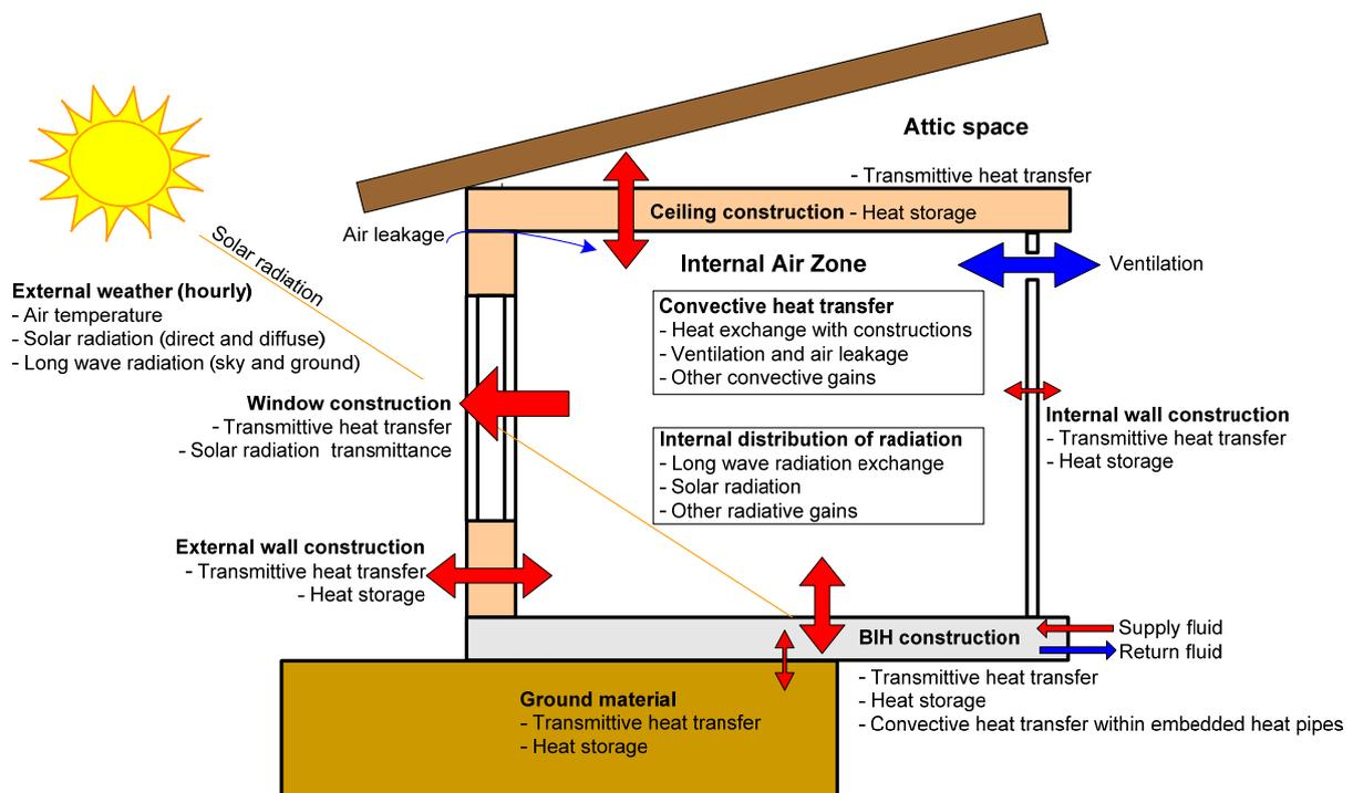
Figure 14 Schematic flow diagram for the general thermal problem with BIH. (Karlsson, 2006)
