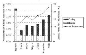
Figure 8 Energy reduction rates by changing preset temperature and annual mean air temperature
