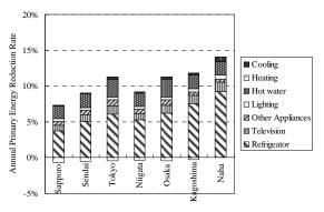
Figure 5 Energy reduction rates by improved energy efficiency of appliances
