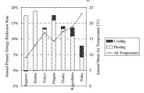
Figure 7 Energy reduction rates by improved heat insulation and mean annual air temperature
