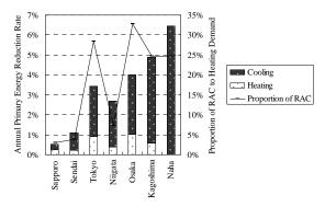
Figure 6 Energy reduction rates by improving rated COP of RAC and proportion of RAC to heating demand
