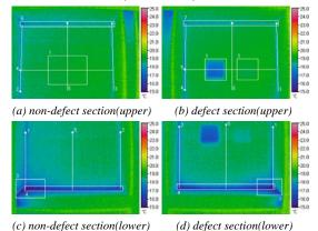
Figure 17 Infra-red thermal imaging data Table 4 Mean surface temperature & TDRi
