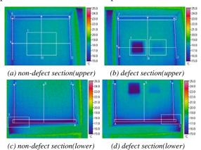
Figure 14 Infra-red thermal imaging data Table 3 Mean surface temperature & TDRi
