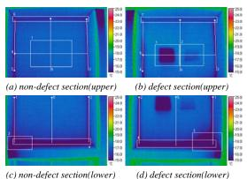
Figure 11 Infra-red thermal imaging data Table 2 Mean surface temperature & TDRi
