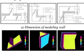
b) Thermal conductivity of modeling wall Figure 1 Simulation subject wall for pattern analysis
