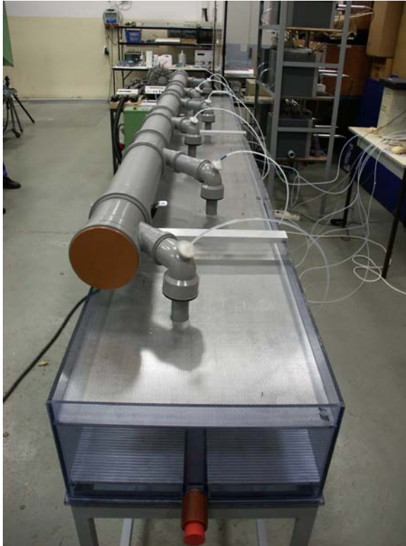
Figure 2 “Emission model” for investigation the influence of different versions of ventilation systems on the emission behaviour of a compartment for fattening pigs
