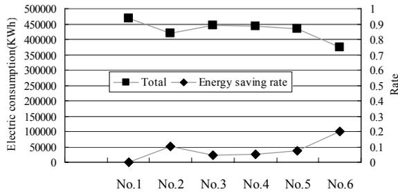
Figure.6 Building Energy Consumption & Energy Saving Rate
