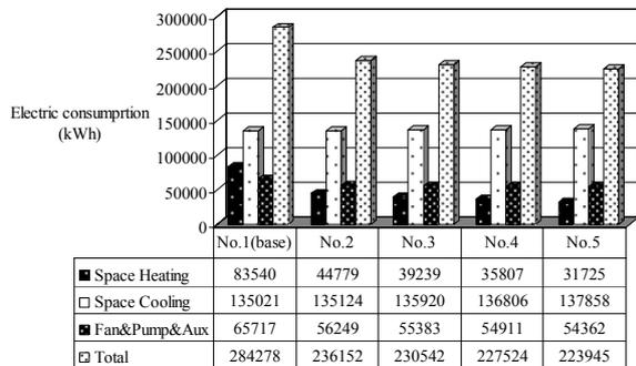
Figure.2 HVAC System Energy Consumption of different "thermal insulation" measures
