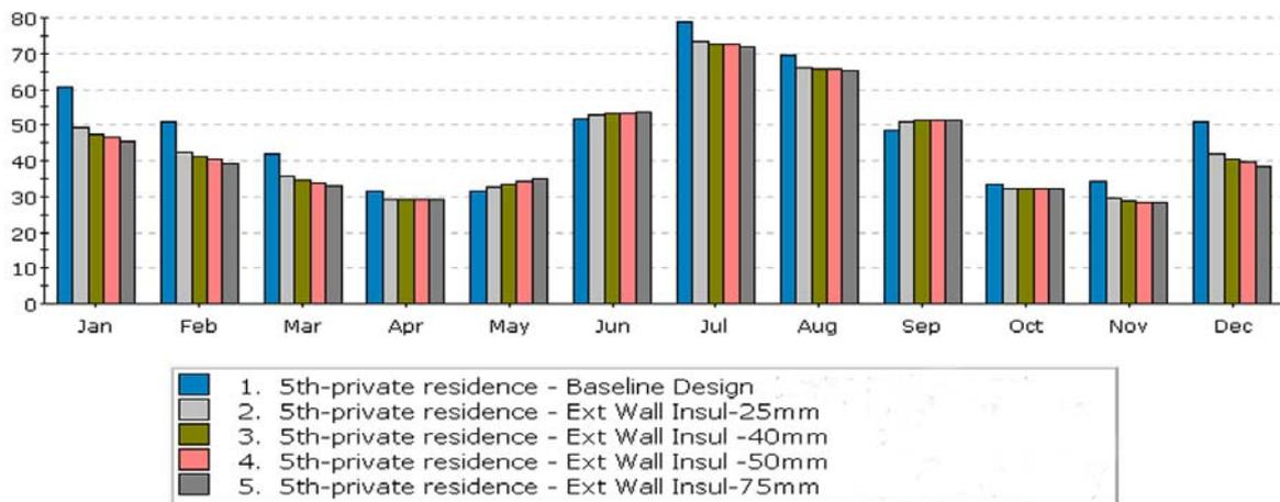
Figure.3 Monthly Total Energy Consumption(KWh)
