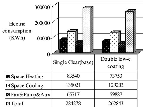
Figure.4 HVAC System Energy Consumption of different “window glass type” measures
