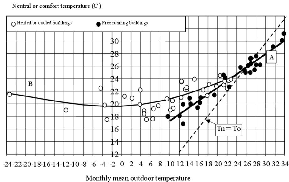
Figure 3 : The change in comfort temperature with monthly mean outdoor temperature for free floating and air conditioning buildings, (From Nicols 2003)
