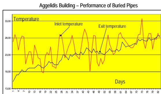
Figure 10: Inlet and outlet temperatures in one of the heat exchangers during the summer period
