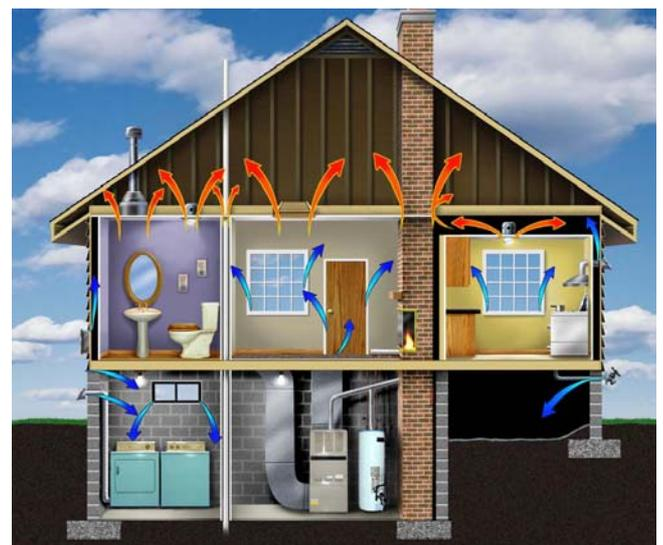
*Figure 1: Uncontrolled air leakage, known as air infiltration, across the building envelope of a house.<sup>1</sup>*
