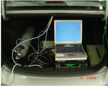
Figure 7. Measurement method of indoor air in a car at drive mode
