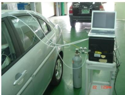
Figure 6. Measurement method of indoor air in a car at stop mode
