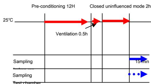
Figure 4: Measurement schedule of indoor air quality in a car (Korea)
