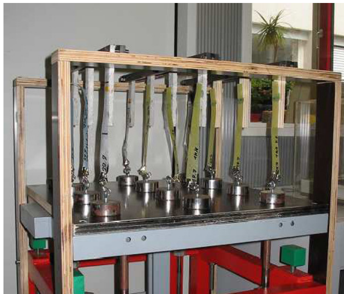
Figure 9: Apparatus developed in Germany to test the durability of adhesives under alternating loads. Each tape is attached to weight that periodically puts the tape under stress (see Ackerman, 2012).
