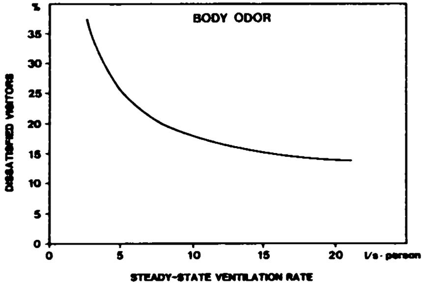
**Fig. 5.2: Percentage of dissatisfied visitors as a function of calculated steady-state ventilation rate. The figure applies for a mixed group of females and males.**
