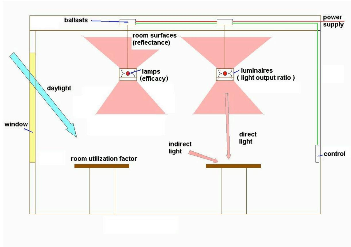
Figure: different sections of a lighting installation.
