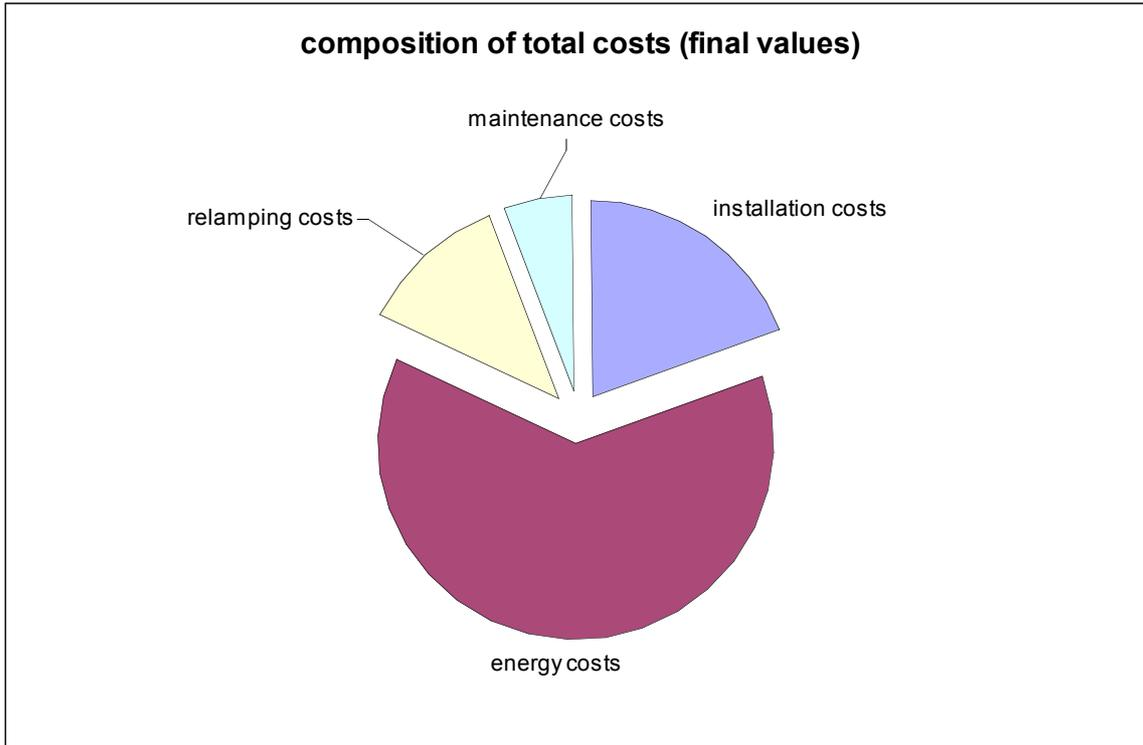
Figure: life cycle costs (dimensions) for a typical store lighting (non-daylit area).
