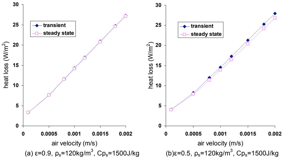
Figure 4: Heat loss under different heat capacity condition
