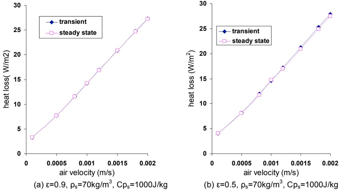
Figure 3: Heat loss obtained under steady-state and transient condition
