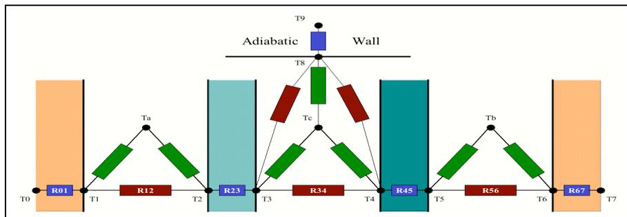
Figure 2: Original delta network for the three-zone simulation
