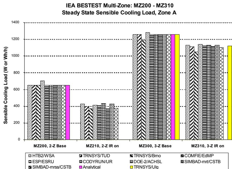
Figure 1: MZ-200 case: comparison of TRNSYS Type 56 with other programs
