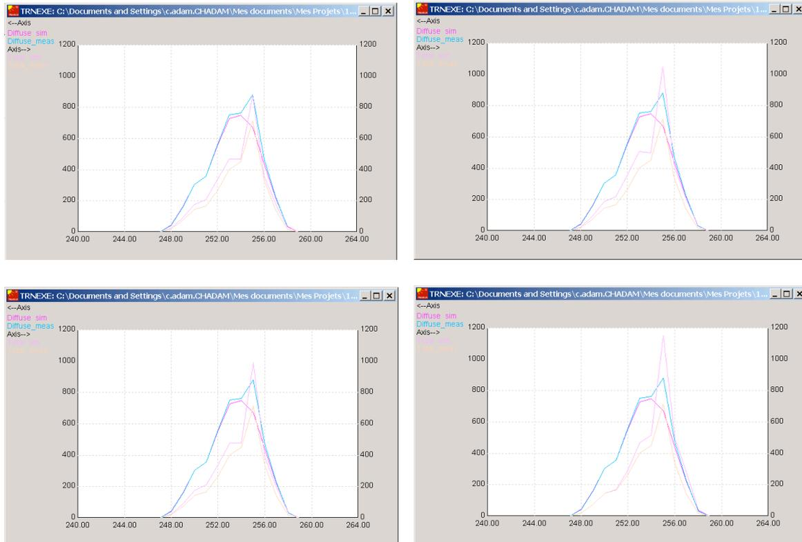
Figure 5: comparison between measured and calculated total radiation on vertical façade for 4 tilted surface radiation modes (upper left: isotropic; upper right: Hay and Davies; lower left: Reindl; lower right: Perez)
