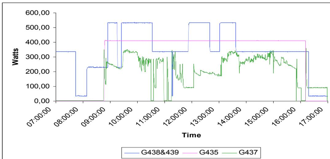
Figure 1: Power consumption curve for rooms G435, G437, and G438&439
