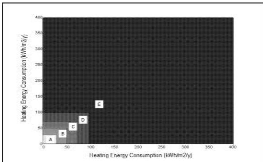
Figure 7 Defined energy classes of heating energy consumption for school buildings in Greece when equal frequency techniques are applied
