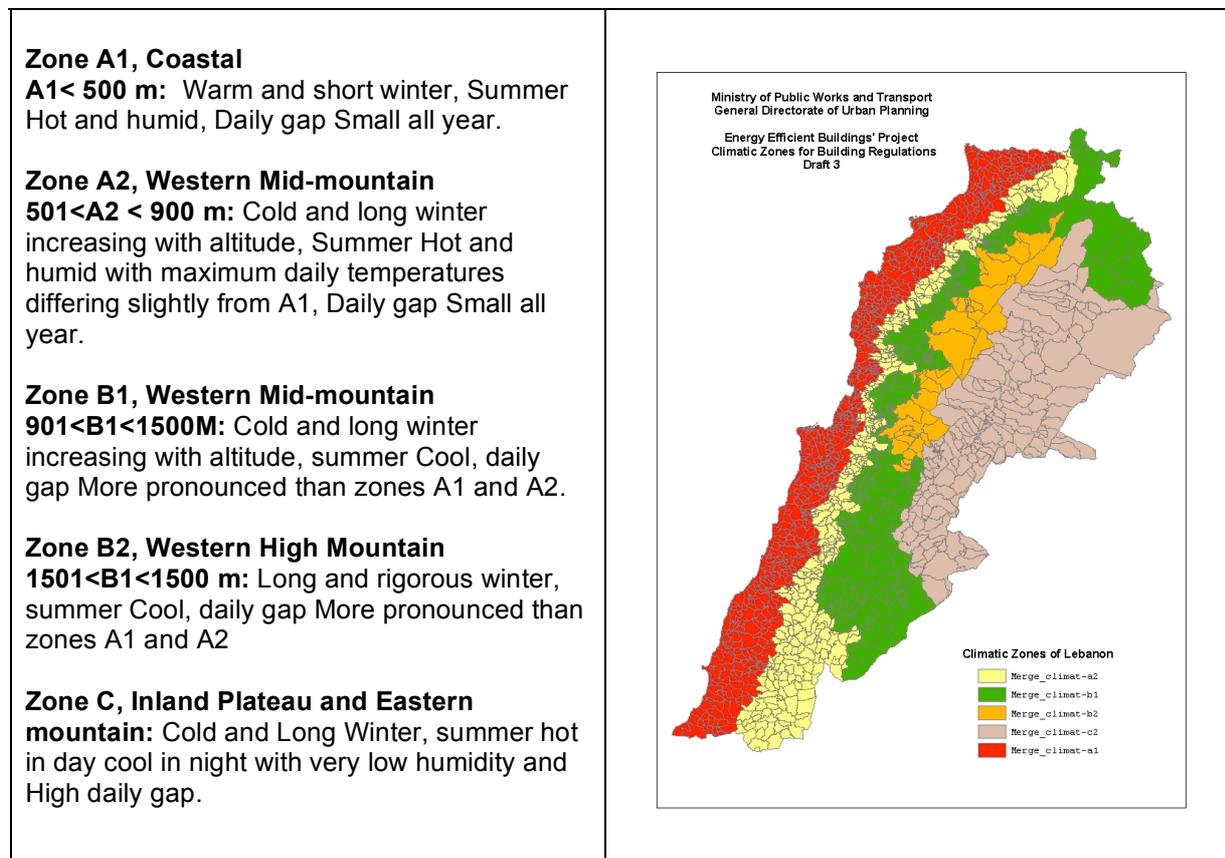
Figure 1: Climatic Zones for Thermal Standards for Buildings in Lebanon
