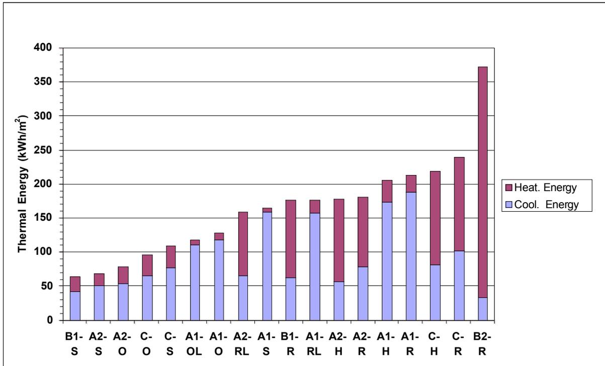
Figure 2: Specific Thermal Energy needs (Heating and Cooling) per year for Base Case Buildings before corrections (kWh/m<sup>2</sup>.year)
