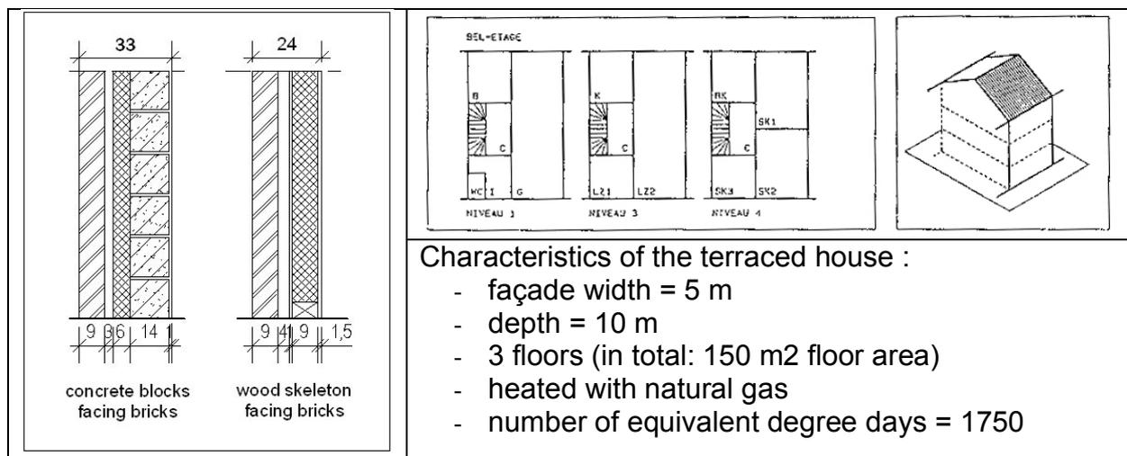
Figure 2: Two compared exterior walls (left) and terraced house (right).
