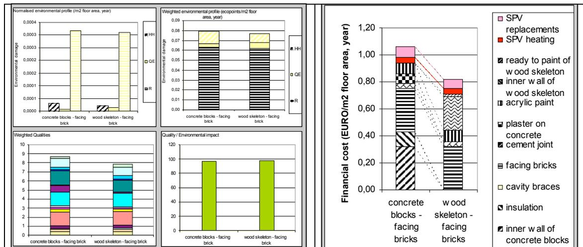
Figure 4: The EI (left) and financial cost (right) of the walls with 14 cm insulation.
