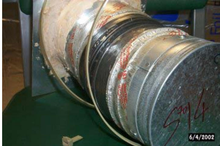
Figure 14. The failed plastic strapping on one of the flexible core to sheet metal collar specimens after four months of aging.
