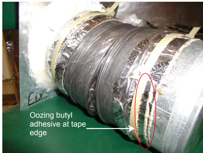
Figure 13. Oozing of the adhesive layer in the foil-butyl tape (Tape 4) specimens (showing result of 5 months of aging).
