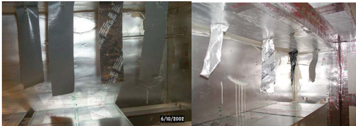
Figure 10. Hanging specimens of Tapes 1 to 4 in the high temperature baking apparatus before testing (left) and after three weeks of testing (right).
