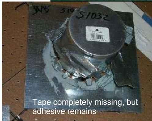
Figure 21. Example failures of the collar-to-plenum joint.
