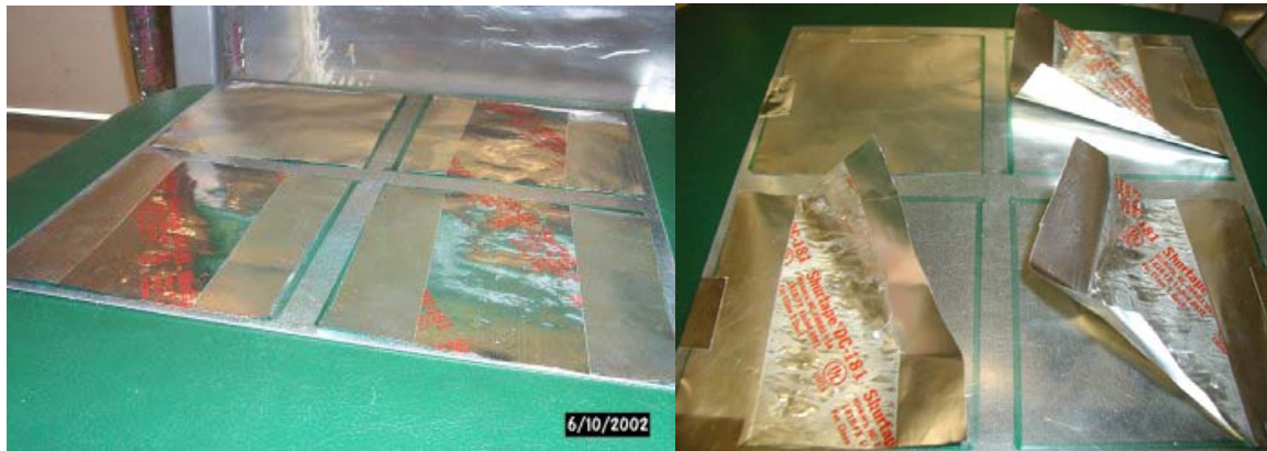
Figure 9. A baking specimen following the UL 181B temperature test protocol consisting of three samples of tape (Tape 3) and one control sample of the substrate (Aluminum Foil) before testing (left) and after four weeks of testing (right).
