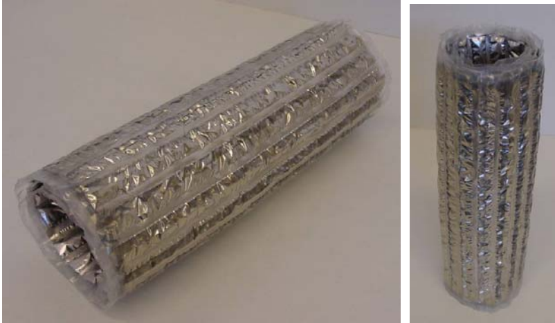
Figure 2. Sample GFP duct section using longitudinal seams and concentric tubes (Photo: Goudey, LBNL)
