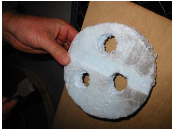
Figure 8. Flow mixer added to Phase 2 apparatus to increase mixing within the duct
