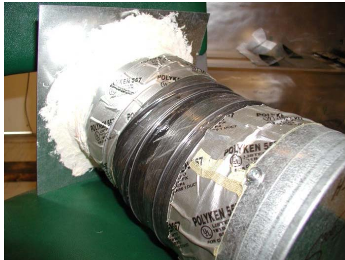
Figure 10. Shrinkage and delamination among the unclamped specimens (showing here result of 5 months of aging)
