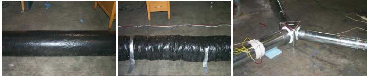
Figure 1. Stretched and compressed 10" (250 mm) flexible duct and splitter box test specimens.
