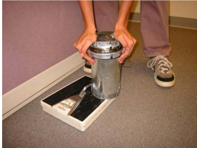
Figure 1. Pressing together the adjustable PEGIT duct fitting on a scale
