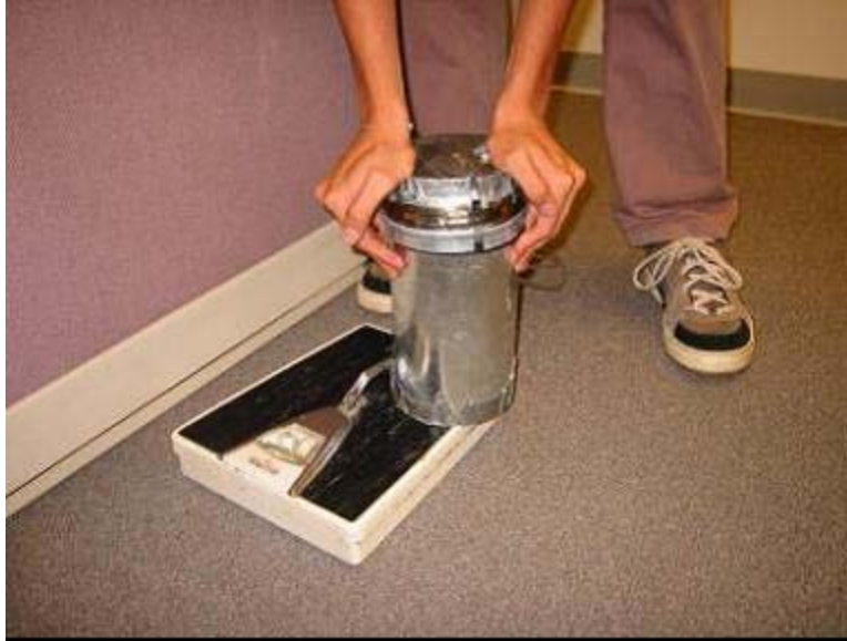
Figure 5. Assembly force measurement using a scale
